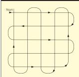
The Random Orbital keeps the pad rotating in an orbit as it's spinning so you can't over-polish your paint. Just maneuver the machine in a cross-hatch grid pattern, shown in the accompanying diagram.
