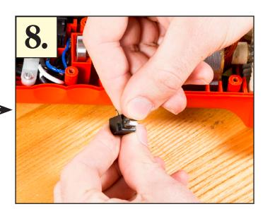
• Installation is the reverse of removal. Make sure to align the groove in the new brush with the tab that is in the plastic housing. Press the carbon end of the brush into the plastic housing and reinstall the plastic housing into the tool case
