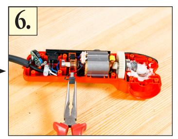
• Use the flathead screwdriver or needle nose pliers to carefully slide the plastic brush housing up away from the tool case.
