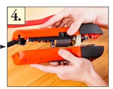
• Once the case starts to come apart you can either continue to carefully use the tool or use your hands to completely separate the two halves of the case.
