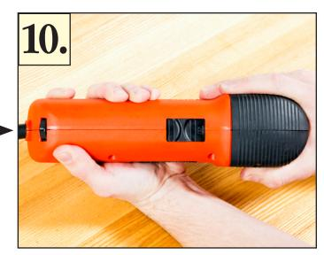
• Double check that everything is installed correctly and carefully re-assemble housing halves together. Once they are aligned, use your hands to carefully "snap" the two halves together.
