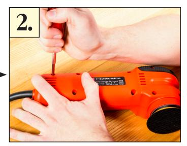
• Using a #2 Phillips head screwdriver remove the ten Phillips screws from the body of the orbital.
