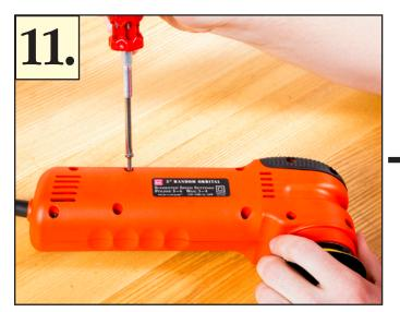
• Re-install and tighten the ten Phillips screws securely. DO NOT OVER TIGHTEN!
