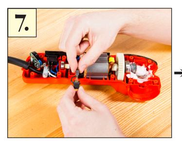
Holding the plastic housing with one hand remove the brush from the housing by carefully pulling on the carbon end. It may require wiggling the brush end to free it from the housing. The brush has a spring that is attached to the bottom.
