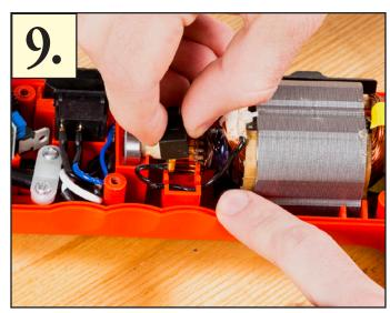
• When re-installing the plastic housing with the new brush make sure to insert the wire in the appropriate grooves
