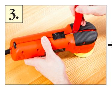
• Use a plastic pry tool (preferred) or small flat head screwdriver to carefully pry open the casing.
