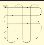
The Random Orbital keeps the pad rotating in an orbit as it's spinning so you can't over-polish your paint. Just maneuver the machine in a cross-hatch grid pattern, shown in the accompanying diagram.
