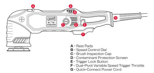
**WARNING:** Never modify the power tool. Damage or personal injury could result.
