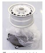
The easiest way to paint a wheel is to place it on a plastic-covered Pneumatic Sit-On Creeper and gently spin the wheel as you paint.
