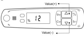
3 When the desired tolerance value is reached, press % to save the value.
