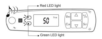
• When applied torque exceeds the wrench full-scale capacity, the GREEN & RED lights will illuminate and the buzzer will continuously beep. The display will read "---".
