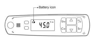
When the battery capacity has only 10% left the battery icon will be displayed. The unit will not work and the batteries will need to be replaced.
