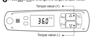
When the target torque value is reached, press SET to save the value.
