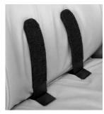
The correct position of brackets inserted into the seat. (Shown without Heated Lumbar Support attached.)
