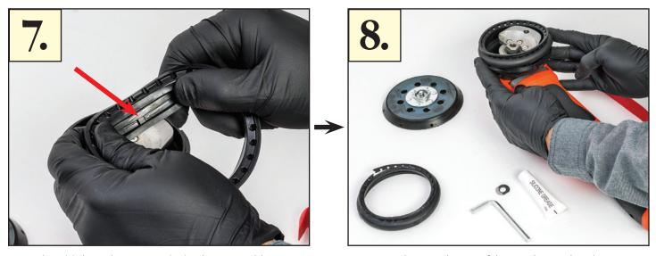
Once the old shroud is removed take the new rubber shroud and locate the tabs around the inside of the shroud.
