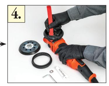
Using your hands, carefully pull the rubber shroud back from the plastic housing and insert your trim removal tool or pry tool here.
