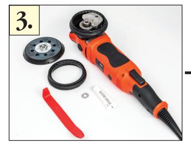
Set the backing plate, stud, and lock washer to the side in a safe place so they do not get lost.
