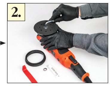
Using the 6mm Allen wrench, hold the backing plate with one hand and unscrew the backing plate stud with the wrench in a counter clockwise motion.
