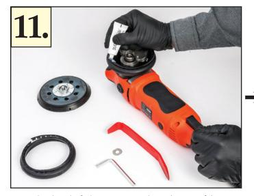
Run a thin bead of silicone grease along the rim of the shroud that will contact the backing plate.
