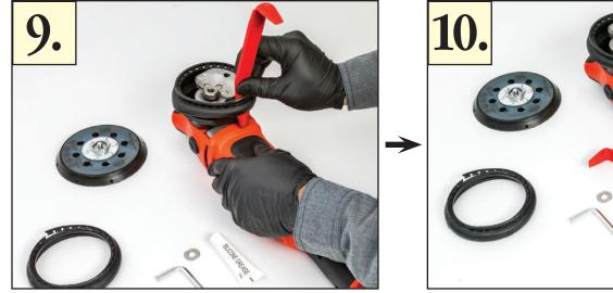
With the tab and notches lined up, begin working the new shroud onto the plastic housing. Once the shroud is about half way on, use your trim tool to stretch the rubber shroud securely around the entire plastic housing.
