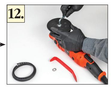
Spread a thin layer of silicone grease over the top surface of the backing plate (side opposite of the Velcro) and re-install the backing plate onto the tool hub using the stud and lock washer that you removed in step 2.
