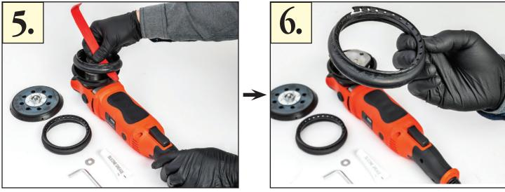
With the trim removal tool placed between the rubber shroud and plastic housing, carefully slide the trim tool through the seam around the entire shroud, releasing it from the housing.
